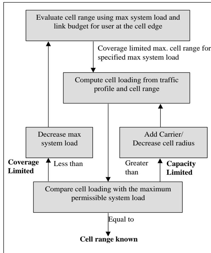
Figure 2 – The process used for system dimensioning
