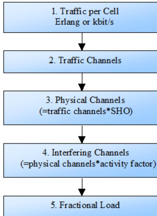
Figure 3 – The process used for system dimensioning
