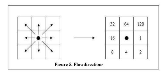
The flow direction grid can be computed by the active DEM region using a custom version of the TOPAZ model distributed with Geographic Information System [7]. The flow direction grid is then imported as a DEM point attribute, and is used to define the flow regime of the entire domain as illustrated in Figure (6) below.
