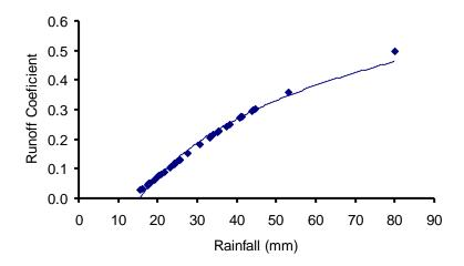
Figure (8): Rainfall depth and Runoff Coefficient relationship.
