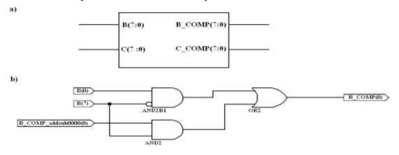
Figure (10): COMP unit a) block diagram .b) gate-level for two-complement form of 1-bit.
