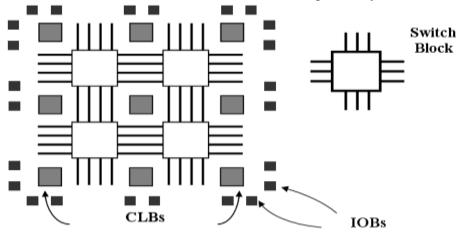
Figure (2): The structure of FPGA.
