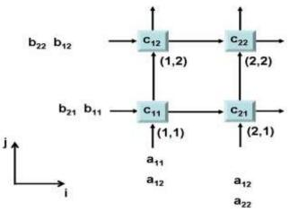
Figure (4): required interconnections between the PEs.
