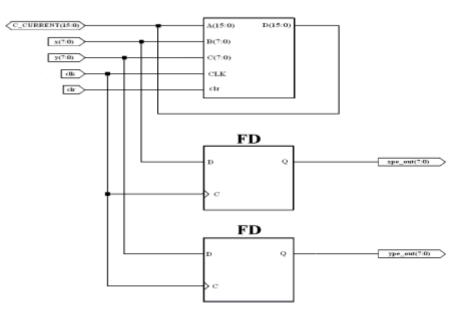
Figure (8): RTL level of PE Architecture.
