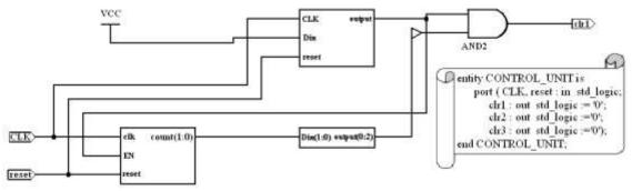
Figure (7): control unit architecture.
