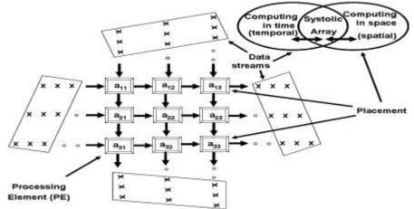
Figure (3): general architecture of systolic array
