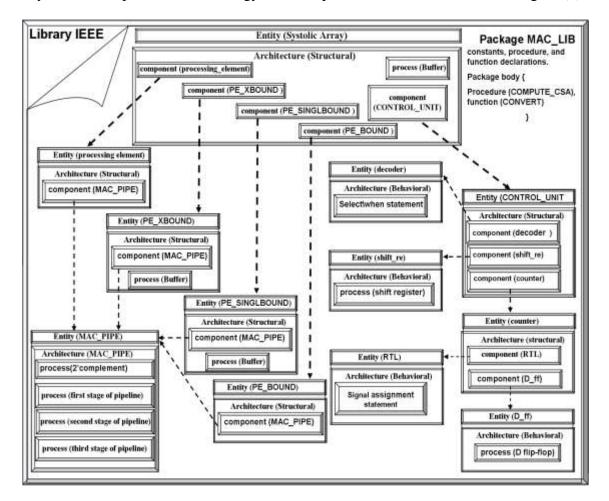
Figure (5): Hierarchical organization of a VHDL design for systolic array based on top-down methodology.
