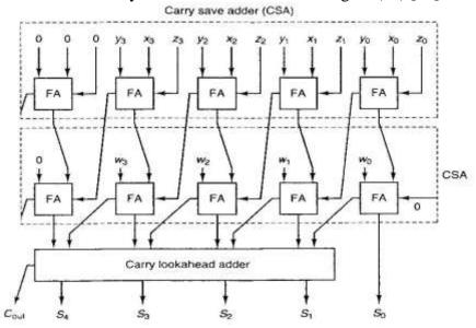
Figure (11): Block diagram of an adder for adding four 4-bit numbers.
