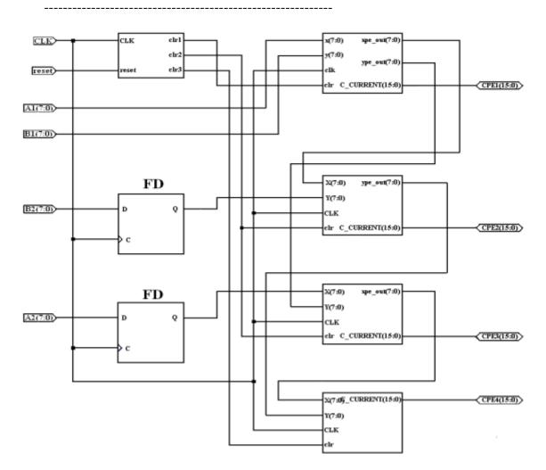
Figure (6): RTL level for 2D systolic array.
