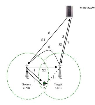
Figure 1: Summary of the different steps of preparation, execution and completion HO process which performs by eNBs.
