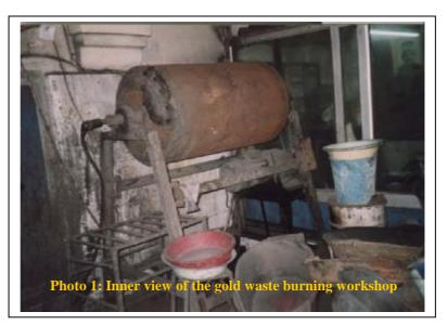
The suggestion is to modify the working process by making the waste combustion internal inside a special fabricated kiln to prevent indoor and outdoor emissions. Emissions of gases will be no more harmful for the neighboring activities and residents thanks to the installation of a filter at the exhaust source.
