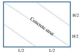
Fig (14) Diagonal compression strut for concrete wall model
