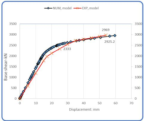
Figure (9) Force- Displacement in experimental and analytical model
