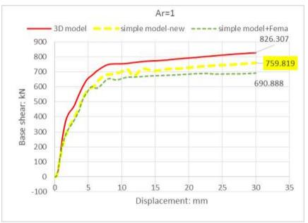
Fig (17) C-SPSW force-displacement in case 3D and simple model by Eq(8) and modify Eq(10)
