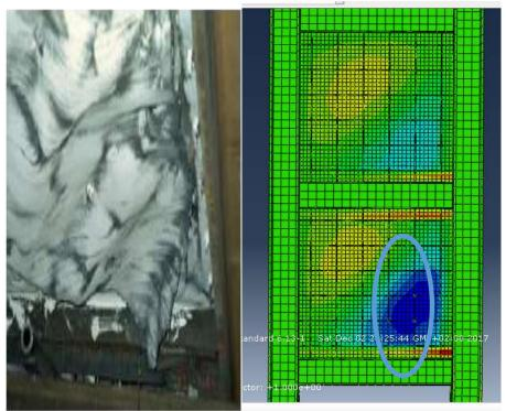
Figure (8) Buckling steel plate in experimental and analytical model
