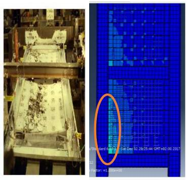
Figure (7) cracking places in experimental and analytical model
