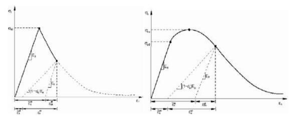
a Parameters for tension model of concrete b-Parameters for compression model of concrete Figure 5. [ABAQUS V6.14 Documentation] [7]
