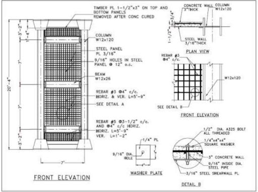
Figure 1. A Specimen with Details of Concrete Shear Wall [5]
