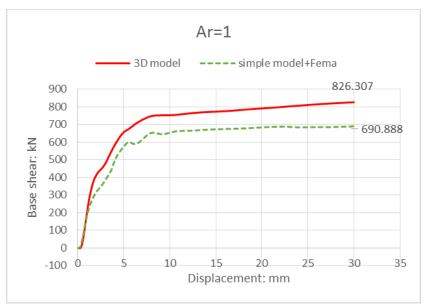
Fig (15) C-SPSW force-displacement in case 3D and simple model by Eq(8) Table (2) summarized the wall specification
