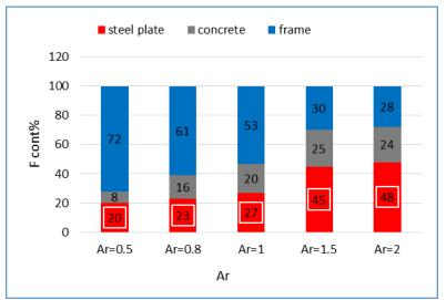
Fig (12) shear force contribution of component C- SPSW with different aspect ratio (Ar)
