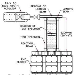
Figure 2. Test Specimen and Test Set-up[5]
