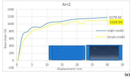
Fig (18) C-SPSW force-displacement in case 3D and simple model by modify Eq(10)
