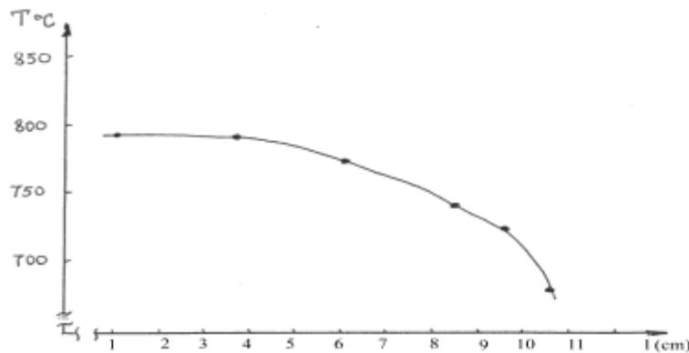
**Figure 1. The measured temperature profile along the axis of the furnace.**
