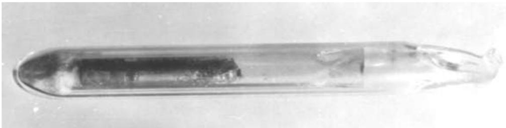
**Figure 6. Quartz ampoule with GaSb Earth analogue.**
