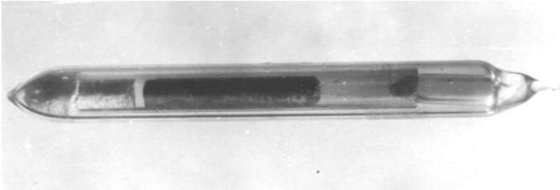
**Figure 5. Quartz ampoule with GaSb Earth analogue.**
