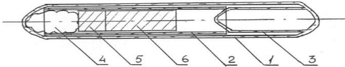
**Figure 3.** The construction of ampoule used in experiment Aphia. 1 is quartz ampoule; 2 is quartz block fitting; 3 is quartz stop; 4 is kaolin wool; 5 is seed and 6 is charge.
