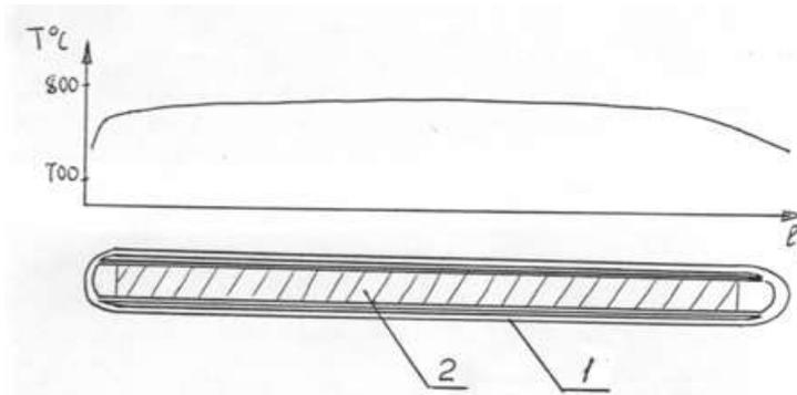
**Figure 4:** The construction of ampoule used in synthesis. 1 is quartz ampoule and 2 is Ga+Sb.
