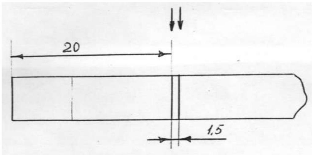
Figure 21. The scheme of the sample cut.
