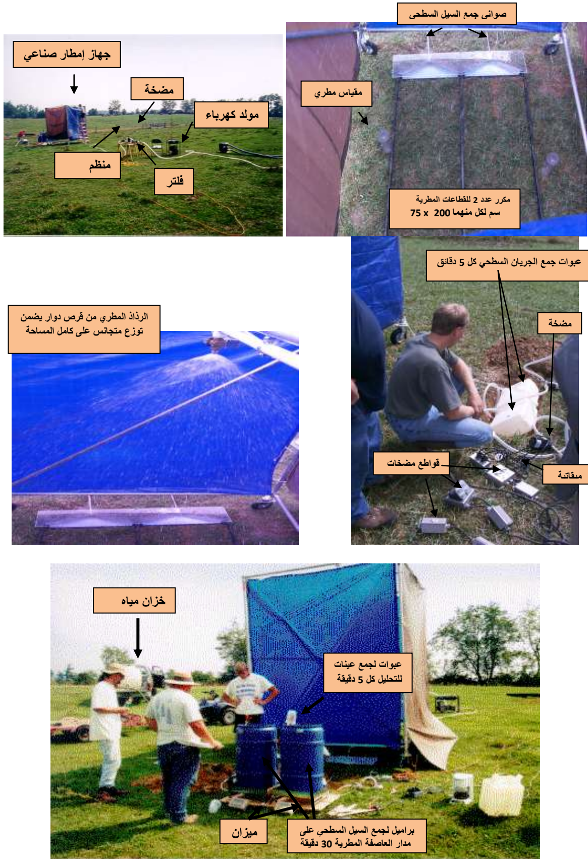
Figure 1: The rainfall simulator used in this study was based on the design of Miller (1987) and experimental procedures were adapted based on the accepted protocol of a national P runoff project (Sharpley et al., 1999).
