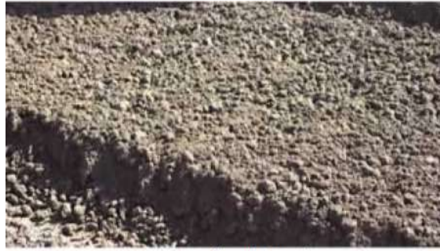
Lime flocculating clay
