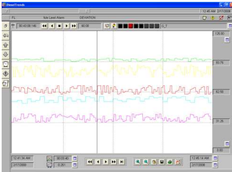
Figure(13): trends page has eight pens, five of which are related to fuel and Coolant level, oil and generator temperature, and engine speed. The sample period of the pens is 1 second.
