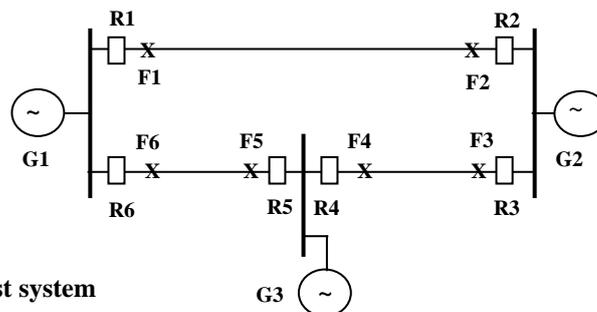
Figure (2) A 3-bus test system
