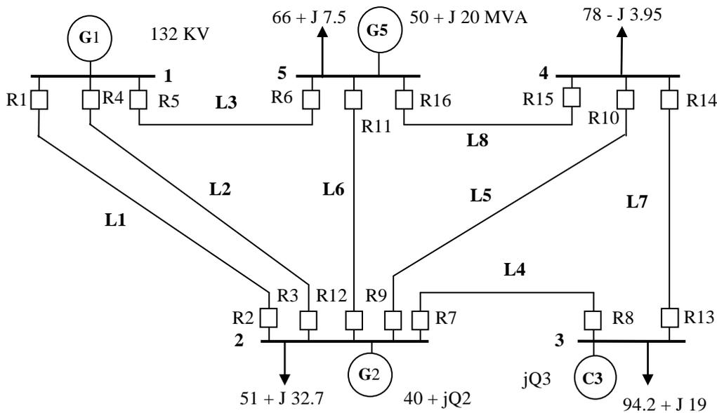
**Figure (3) The IEEE 5-bus test system**
