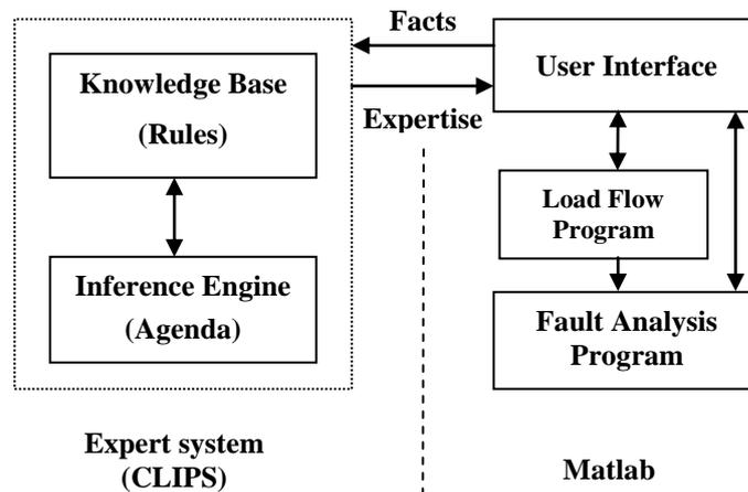
Figure (1) A block diagram for the developed ES based protection coordination.
