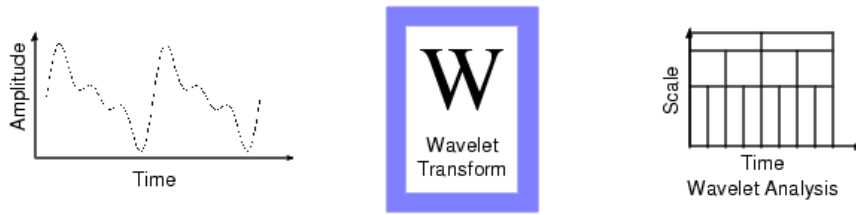
Fig (1) shows the time and scale (frequency) relationship in wavelet transform.
